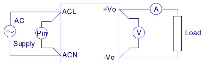
Figure 1. TR60M Series Test Setup
