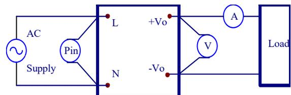
Figure 1. TR30RAM Series Test Setup
