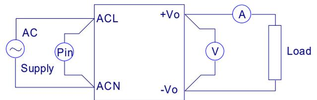
Figure 1. TR220MA/B Series Test Setup
