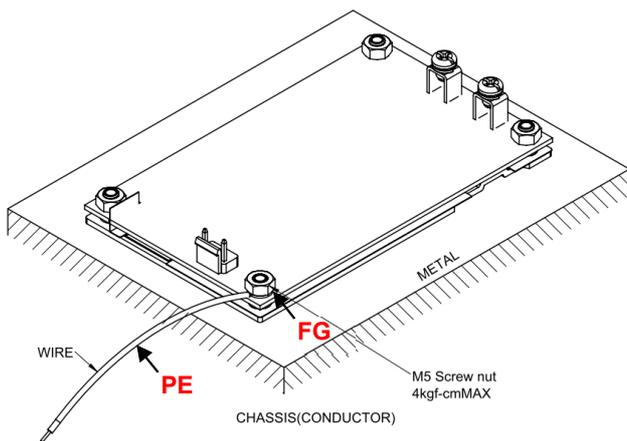
The torque of M5 screw nut is 4kgf-cm.
