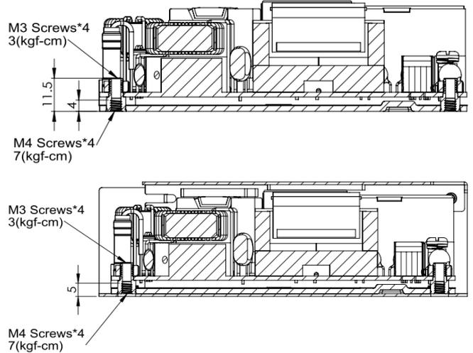
The torque of M3 screws are 3kgf-cm and M4 screws are 7kgf-cm. The torque of output connectors are 7kgf-cm and the connectors mate with round terminal. The maximum outer diameter of the terminal is 8.0mm and the maximum inner diameter is 4.3mm. When locking the round terminal or Y terminal to output connectors, the terminals should not touch other parts to avoid short.
