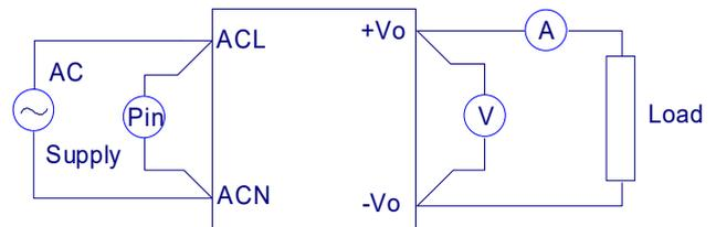
Figure 1. CFM500M Series Test Setup
